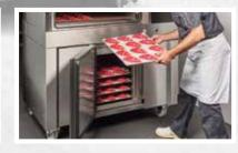
The temperature and humidity can be adjusted according to the products to be proofed in the proof box.
