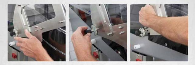
Raise the lid, then gently pull and turn the knobs on either side of the mixer to release it.
