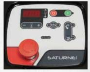
**Electronic control panel with 3 preset speeds** (30, 60 and 125 rpm) and timer. The user can either run the mixer continuously, or set the timer to stop the cycle after a specified duration.
