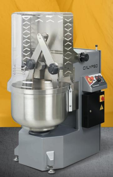
FRENCH BAKERY **EQUIPMENT MANUFACTURER**  **CALYPSO** is a twin-arms mixer that perfectly reproduces the artisan's manual movement by gently kneading the dough to promote its oxygenation and limit heating.
